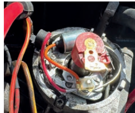
Having inadvertently dropped and lost the retaining nut, Chris was delighted to find that the improvised plastic washer was a tight enough fit on the post to stay in position for the rest of the drive home.
