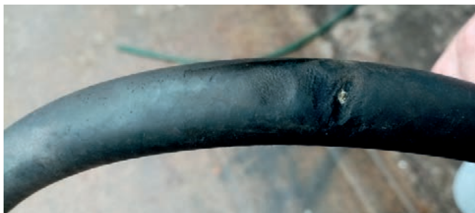
8. Old pipe damaged by steering column joint.
