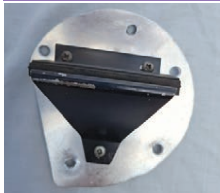
The whole assembly was then fixed to the tunnel using self-tapping screws and spire nuts.
