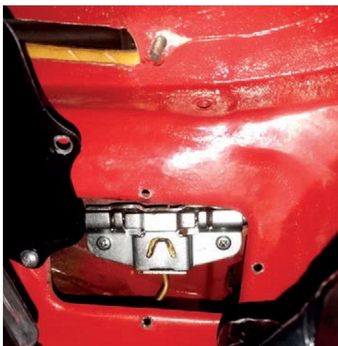
1. Passenger side wiper wheelbox exposed.
