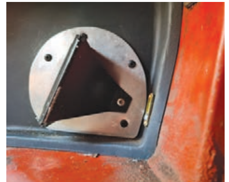
I then straightened the floor section flanges and installed the tunnel using the new fixing kit...
