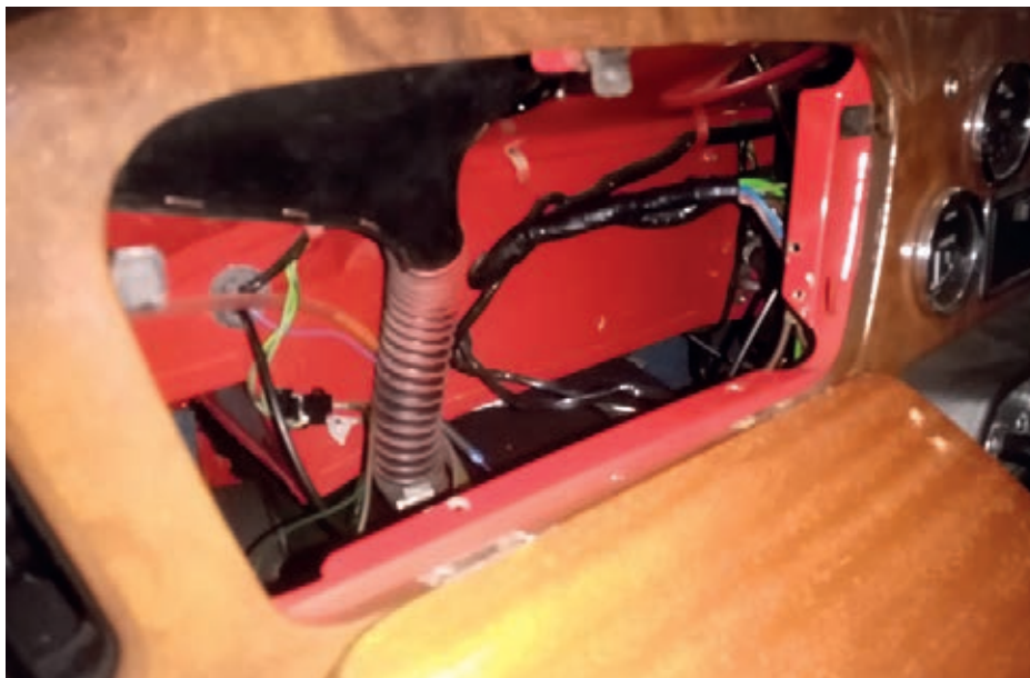
4. Good access with glove box removed.
