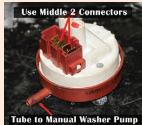
2. There are four male spade terminals on the pressure switch, but on this model you're only interested in the two centre ones. Take your ignition-switched 12v feed and connect to either of the centre two terminals. Run a second cable from the other centre terminal to the positive side of the electric washer pump. The other connector on the electric washer pump should go to ground.
