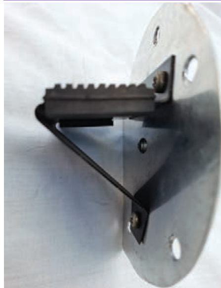
I then cut a piece of 2mm aluminium sheet to fit the corner profile of the tunnel. I fixed the cut out piece to the sheet using the centre hole and three nuts and bolts which secure the foot rest.
