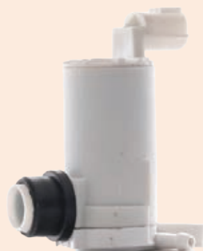
Cut a hole in your washer bottle and use one that fits through the bottle.
